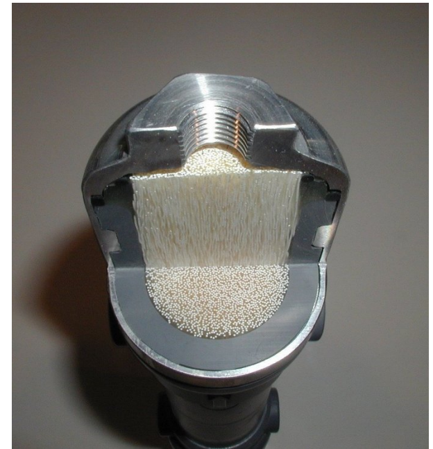
Cut-away of Membrane unit internally packed straws
